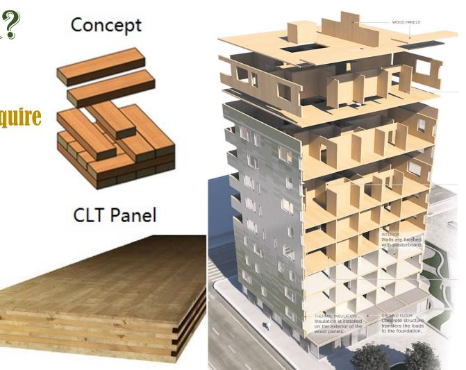
Use CLT panels and the main structural components, walls and floors of the building. 6
