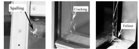
Figure 4: Typical glass damage progression at the corners of insulating glass units constructed with annealed monolithic glass panes with picture (a) showing spalling; (b) cracking; and (c) fallout. 19
